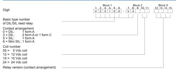
Ordering example: V23100-V4005-A010 DIL reed relay with 1 make, 5 V nominal voltage, with clamping diode (spark suppression)
